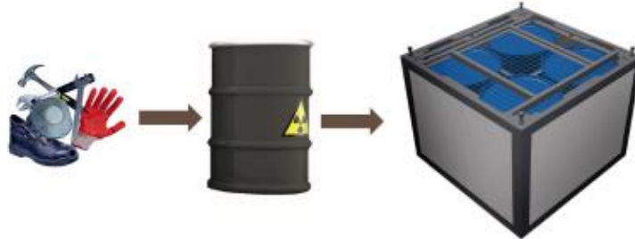
Figure 4.3.1-2. Compact waste package formed with a steel container
