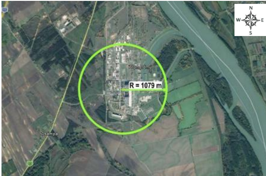
Figure 5.1.2-1. Assumed air quality impact area of the Paks Nuclear Power Plant operation
